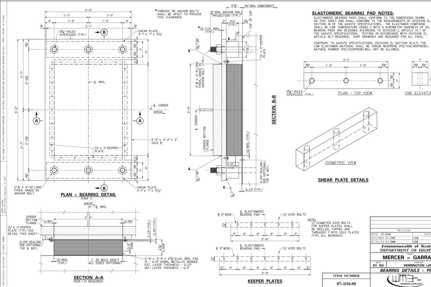
SECTION 18 OF THE AASHTO SPECIFICATIONS. THE ELASTOMER COMPOUND SHALL BE LOW TEMPERATURE GRADE 3 WITH A DUROMETER HARDNESS OF 50. BEARING PADS ARE DESIGNED ACCORDING TO DIVISION I, ARTICLE 14.7 OF THE AASHTO SPECIFICATIONS. TESTING IN ACCORDANCE WITH DIVISION II, ARTICLE 18.7 REQUIRED. SHOP DRAWINGS ARE REQUIRED FOR ALL PADS.
